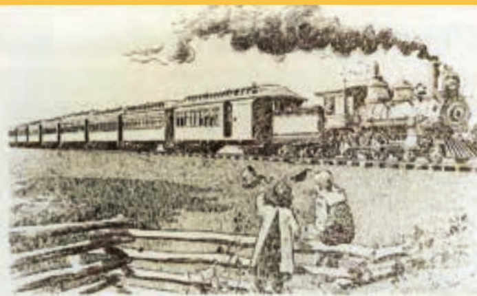
Sketch from a 1898 C. G. & P. brochure. Actually the steam locomotives could not pull more than three cars up the grade of Mt. Washington hill.
