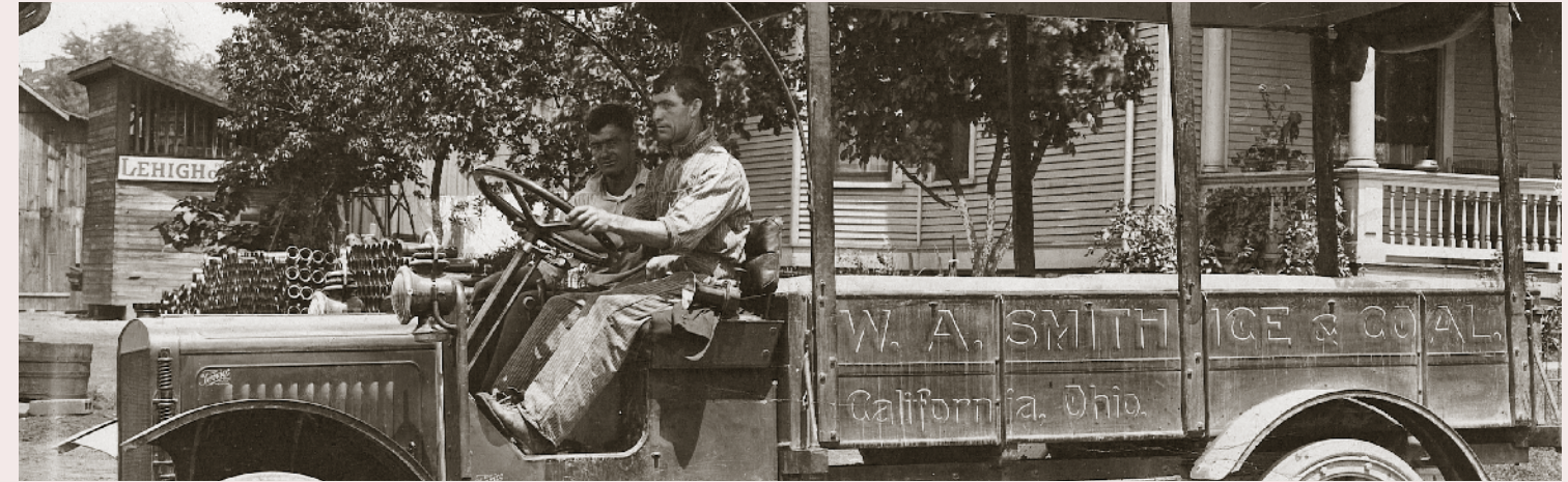
William A. Smith at the wheel of his Ice & Coal Company delivery truck in about 1918. The truck had a chain drive, solid tires and side curtains.
